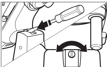
**(OPTIONAL) To adjust beater to bowl clearance:** Tilt the motor head back; then, using a flat-head screwdriver, turn the screw slightly counterclockwise (left) to raise the beater, or clockwise (right) to lower the beater. Adjust the beater so that it just clears the surface of the bowl. If you overadjust the screw, the bowl lock lever may not lock into place.
